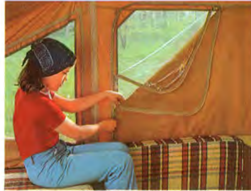
Three way windows include screen, clear vinyl and canvas with zippers. (Curtains replace canvas in some models.)
