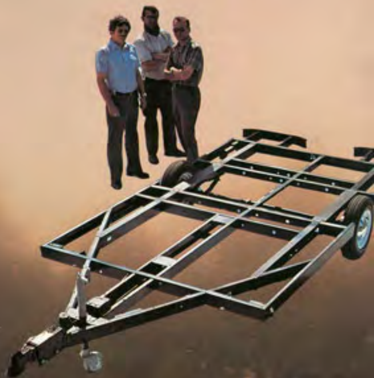
The strongest camper frame made today. Fashioned from 4-inch box channel steel... not 3-inch like most of our competitors use. Structurally reinforced to eliminate bounce and sag. And Starcraft's open perimeter design permits easy tire changes, if you ever need to.
