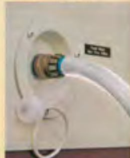
THE STANDARD. Brass city water connector for quick convenient hookup at campsite.
