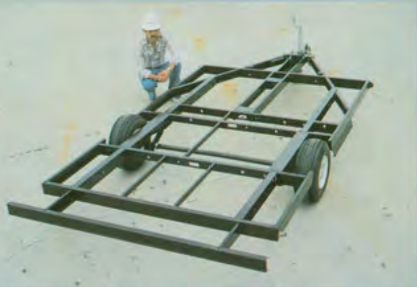
The all new Venture is built on the strongest camper frame made today. It's fashioned from 4-inch box channel steel. Not 3-inch like our competitors use. Structurally reinforced at critical stress points to eliminate bounce and sag.
