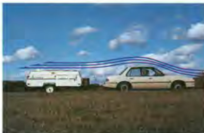
The aerodynamics of the car are really more important than the aerodynamics of the camper. It is the car that interrupts the static air mass. The air then basically flows over the car and camper.
