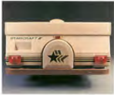
Impact resistant Rovel® endwalls protect Starcraft's luxury campers from damage by flying road debris and are part of the aerodynamic styling.
