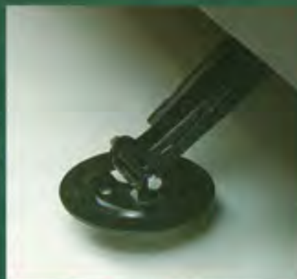
Stabilizing jack with sand pad
