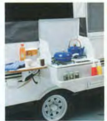
The movable range and work table can be mounted outside for outdoor cooking.
