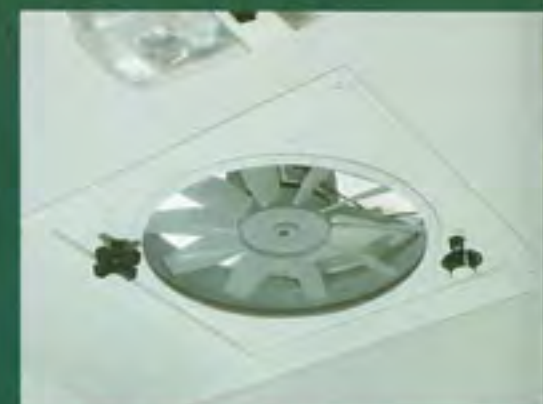
3 speed, 12 volt vent fan dissipates condensation and exchanges the air inside the camper with outside ambient air
