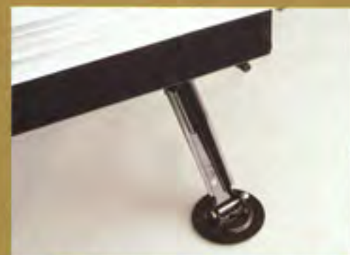
CRANK DOWN STABILIZER JACK WITH SAND PAD
