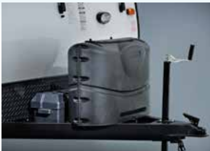
MOLDED LP BOTTLE COVERS (Std. on all Hard Sides and High Walls)
