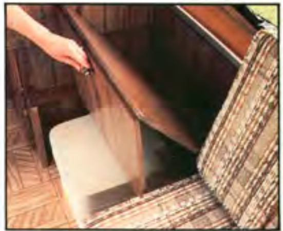
LoneStar has built-in hinged lid chemical toilet storage compartment as standard equipment.
